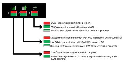
Note 1: The CGW resets itself after receiving new configuration from the server (ex. new HB), LED1 starts with RED and the reset cycle continues till all 3 LEDS are GREEN Note 2: After successful SW upgrade , LED 2 and 3 flash RED then reset cycle starts.
