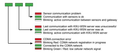
Note 1: The gateway resets itself after receiving new configuration from the server (ex. new HB), LED1 starts with RED and the reset cycle continues till all 3 LEDS are GREEN
