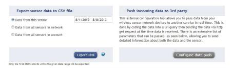
To export sensor data you must first select the date range for the data you want to export. Once the date range is selected, determine whether you want sensor data from the selected sensor only, from all sensors in the network or all sensors assigned to the account. When you are finished, click on "Export Data" at the bottom of this window. The data will be exported to a comma separated value (.csv) file format.
