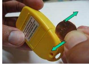
**2. Use coin to remove battery cover. Turn coin *clockwise*. Battery cover will pop off.**
