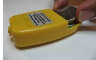
**3. Remove old battery. Wait 10 seconds before inserting new one.**
